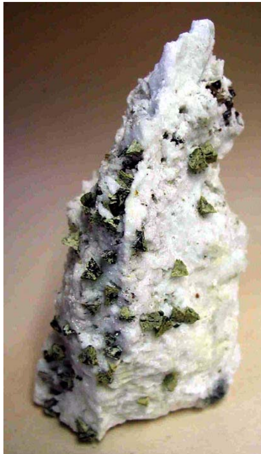
Fig. 1: helvite (greenish tetrahedra to 7 mm) on vuggy albite with acicular remnants of garnet at the upper portion of the specimen, Navegador mine, in Conselehiro Pena, Minas Gerais, Brazil.
