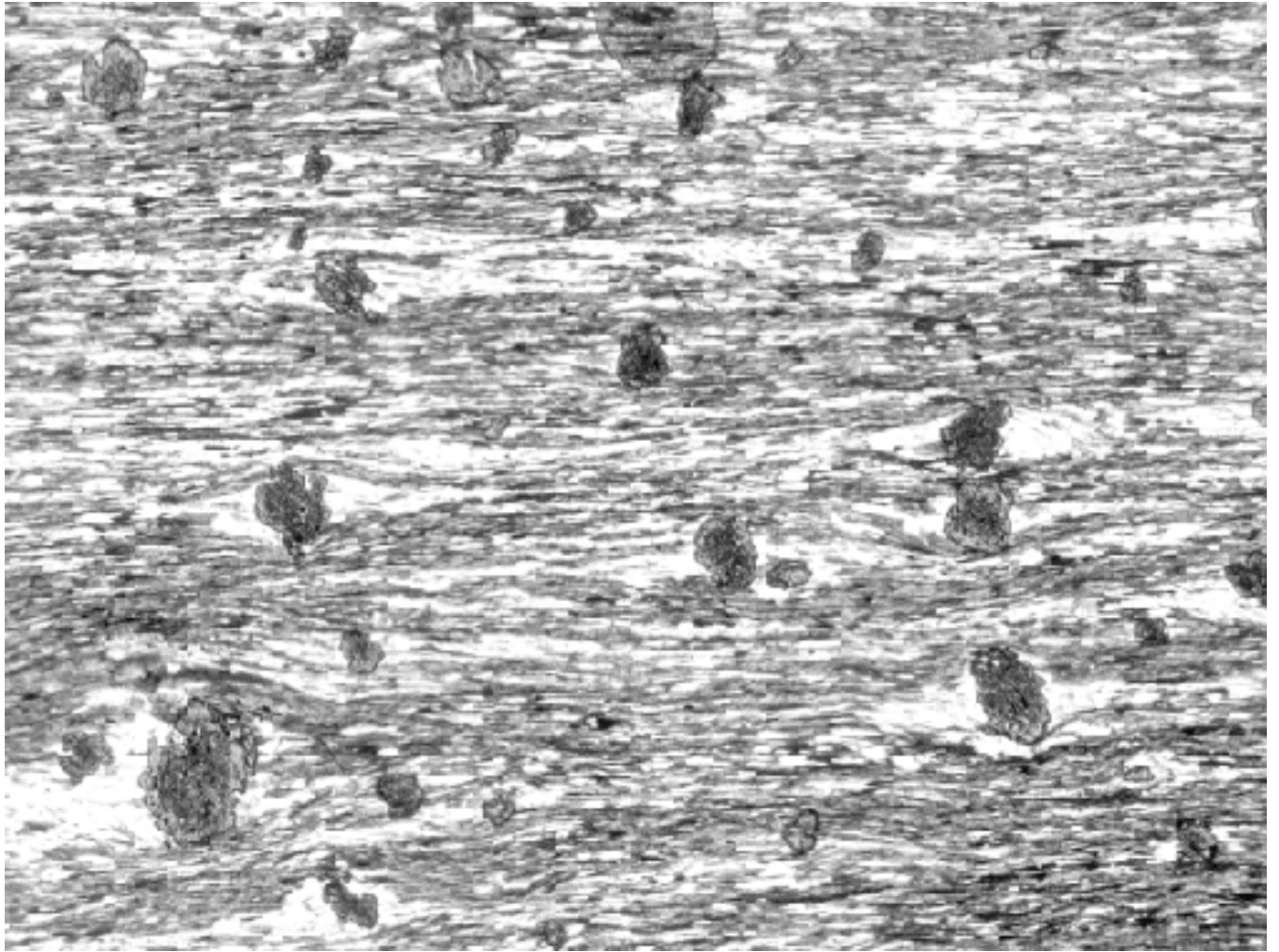
Figure 2. Photomicrograph of sample 96-2. Section is cut perpendicular to foliation and parallel to lineation. Width of field is 6 mm.
